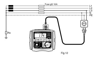
The maximum value of Zs for this example is  $2.1\,\Omega$  (16amp gG fuse,0.4 seconds). The loop tester reads  $1.14\,\Omega$  and consequently the condition Zs<Uo / la is met.
