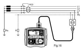
Practical example of 3-phase + neutral RCD test in a TN system
