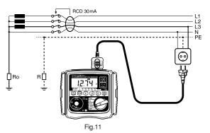
For this example the maximum value is  $1667 \Omega$ , the loop tester reads 12.74  $\Omega$  and consequently the condition RA is  $\leq 50$ /la is met.
